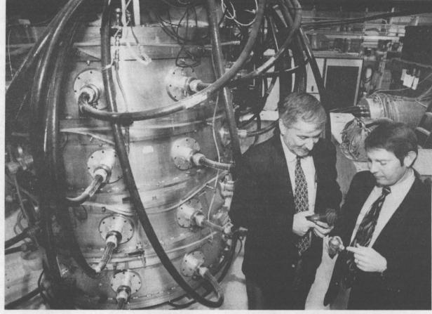
IONS FOR INNOVATION — Gene Neau, left, and Regan Stinnett, next to the RHEPP I accelerator in Area 4 last week, examine an artificial hip joint treated with their ion beam technology. They are the founders of Quantum Manufacturing Technology. (Photo by Randy Montoya)
